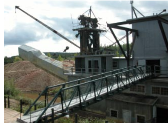
Gold dredge showing gravel conveyor at back
