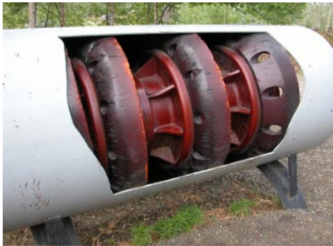
Pig inside cutaway of pipeline
