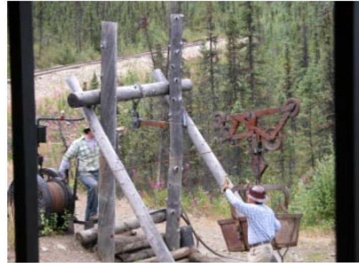
Steam donkey raising bucket of gravel from underground
