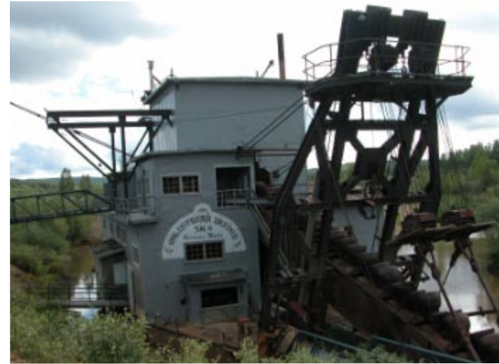
Gold dredge showing bucket line at front
